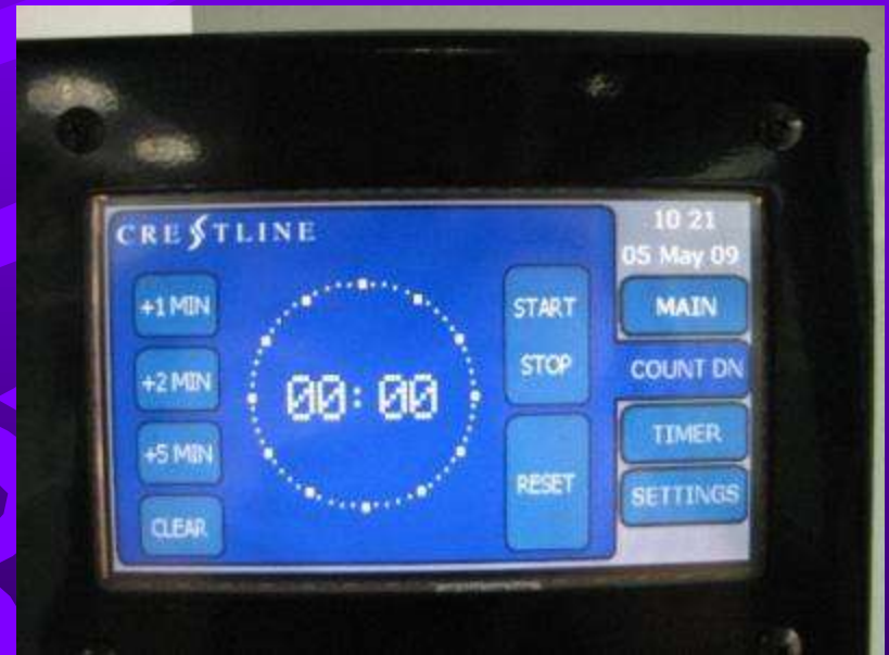
Weldon Multiplex touch screen showing GPS in cab and procedure timer function in patient compartment.
