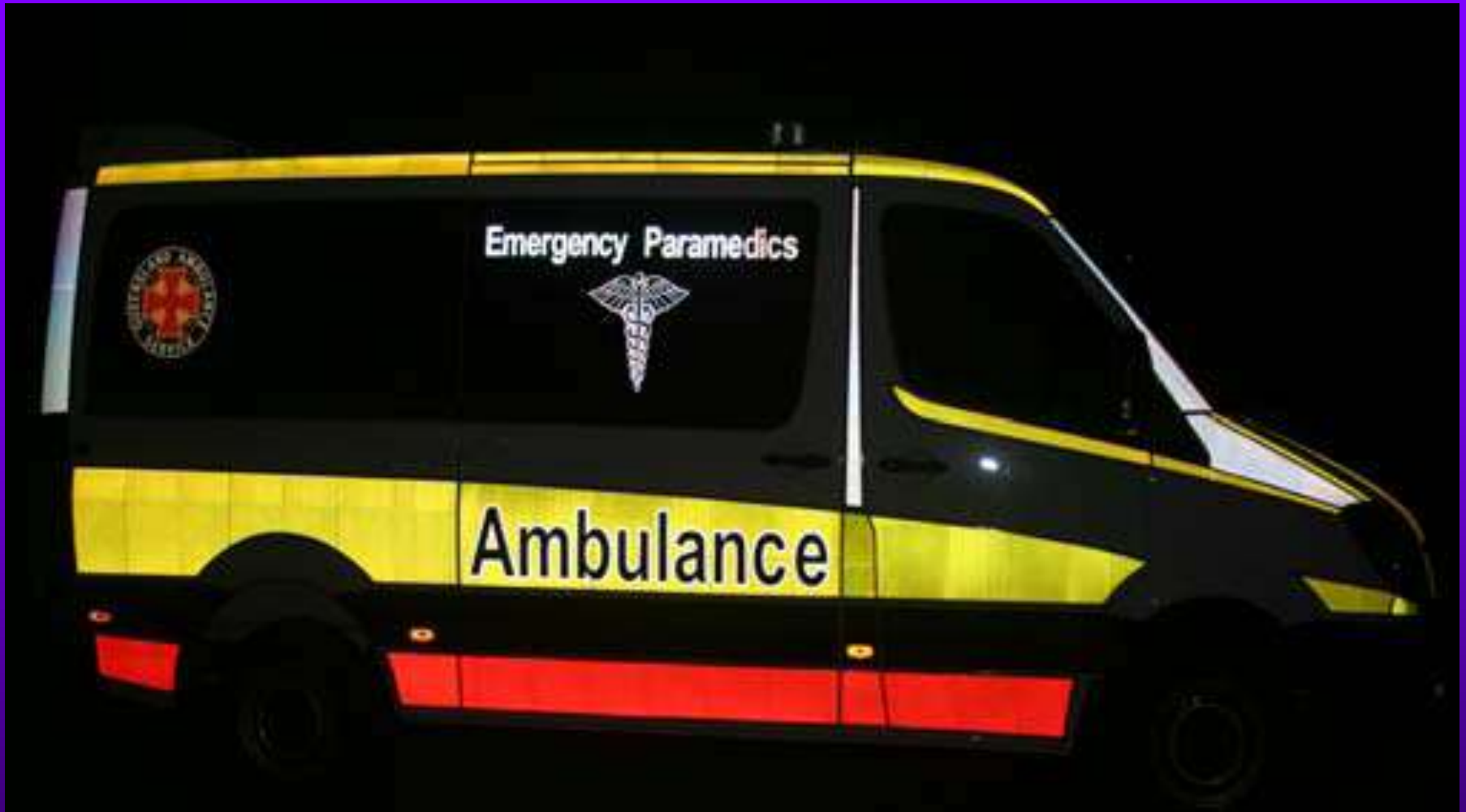
Night time view showing retro-reflective markings
